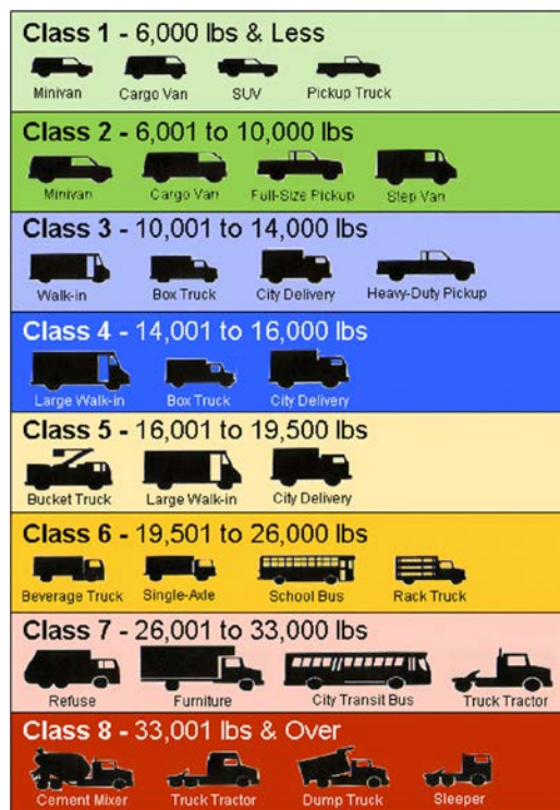
Figure 1. Vehicle weight classes as defined by the Federal Highway Administration, US Department of Transportation (USDOT) Source: US Department of Energy, Office of Energy Efficiency and Renewable Energy webpage
