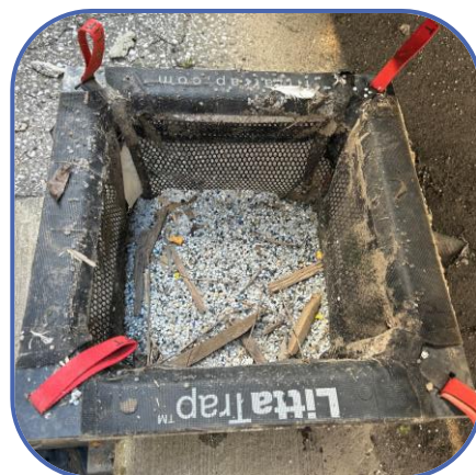
Plastic pellets captured a storm drain screens with a 1 mm liner deployed on the properties of plastic companies.
