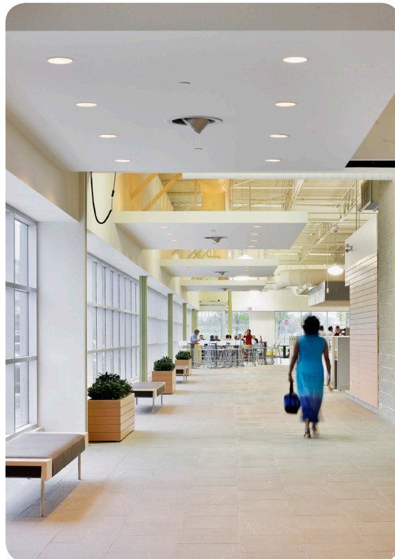
The CHSI Common Area maximizes use of natural light, and includes programmable light fixtures to increase efficiency
