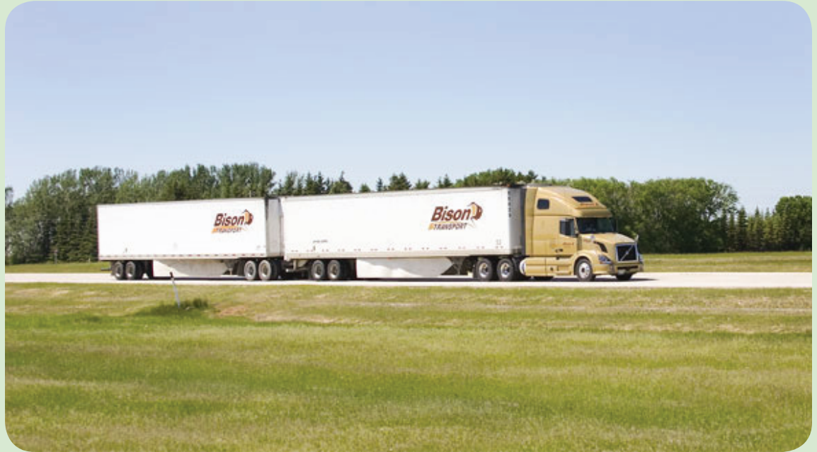
Bison Transport's longer combination vehicles include fuel efficient features such as lightweight trailer skirting and low rolling tires.
