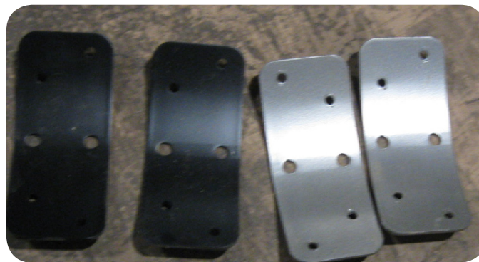
Black furniture pieces on the left were sprayed with new paint, while the silver parts on the right were sprayed with reclaimed paint, saving dollars and resources.
