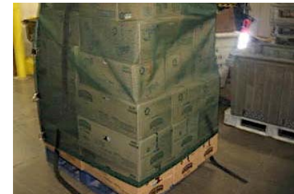
Reusable vinyl wrap is an alternative to plastic film. (Credit: Pallet Wrapz Inc.)
