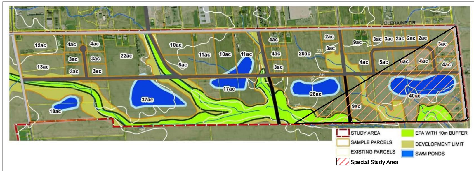
Figure 65. Hypothetical Consolidated Stormwater Management Ponds in Coleraine West Case Study
